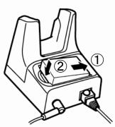
3. Remove the battery from the CU.
