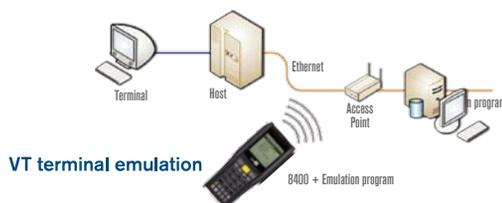
The 8400 is able to emulate terminals VT100, VT220, and TN5250. A bigger, brighter display, function-specific alphanumeric keys and extended battery life bring the power of terminal emulation to the work floor anytime you wish to do so.
