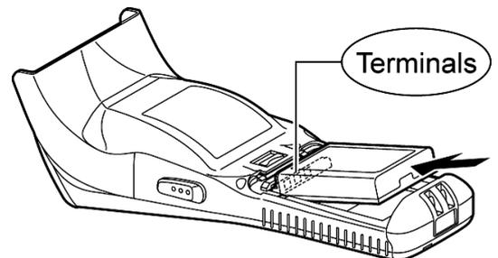
4. Insert the battery cartridge cover tab (1), and then close the battery cartridge cover (2) to lock the cover in position. Press the battery cover into place until a click is heard.
