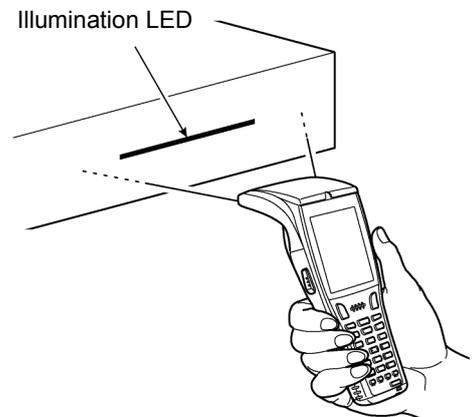
3. Hold the BHT close to the barcode to align the illumination LED.
