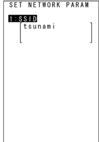
2. Ensure that [1: SSID] is highlighted and press the **ENT** key.
