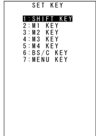
2. Use the cursor keys ([▲] [▼]) or numerical keys ([1] [2] [3] [4] [5] [6] [7]) to highlight the item to be set, and then press the **ENT** key.
