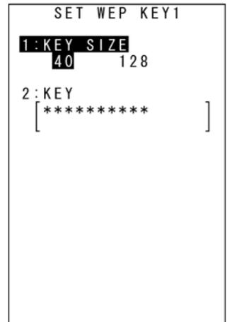
5. Use the cursor keys ([▲] [▼]) or numerical key ([1]) to highlight [1: KEY SIZE], and then use the cursor keys ([◀] [▶]) to select either 40 (40 bit) or 128 (128 bit).
