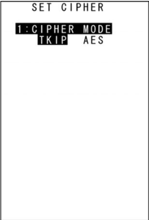
7. Ensure that [1: CIPHER MODE] is highlighted and then select TKIP or AES.
