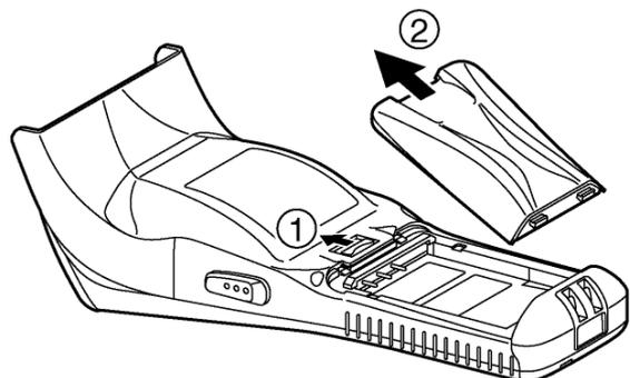
5. Check the battery cartridge terminals and indication on the BHT unit, and then insert the cartridge in the direction indicated by the arrow.
