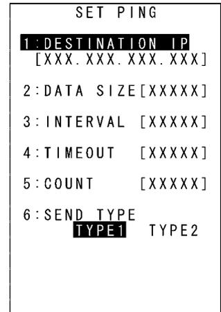
2. Use the cursor keys ([▲] [▼]) or numerical keys ([1] [2] [3] [4] [5] [6]) to highlight the item to be set, and then press the **ENT** key.
