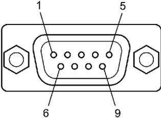
The CU-801 RS-232C interface connector uses Dsub-9P.
