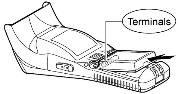
6. Insert the battery cartridge cover tab (1), and then close the battery cartridge cover (2) to lock the cover in position. Press the battery cover into place until a click is heard.
