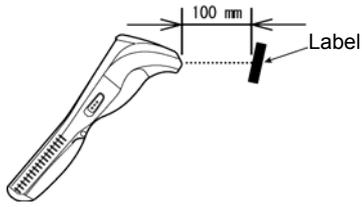
As illustrated at left, align the reading window with the center of the label (code) to be scanned.
