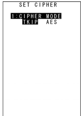
14. Ensure that [1: CIPHER MODE] is highlighted and then select TKIP or AES.
